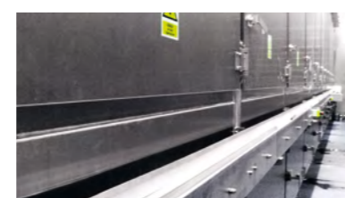
Stick return belt with optional stick cleaning.
