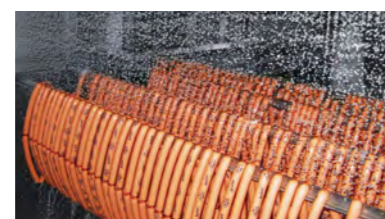
Hygiene protection using a water shower to rinse off sausage particles.
