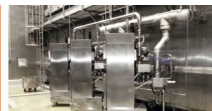
Natural smoke generators with wood chips that can be connected as needed to achieve the desired level of smokiness.
