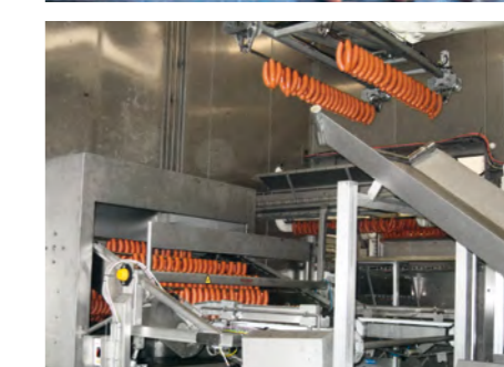
Sausage output ready for direct transfer to packaging.
