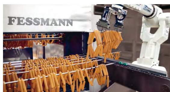
Automatic robot loading from filler to TF4000.
