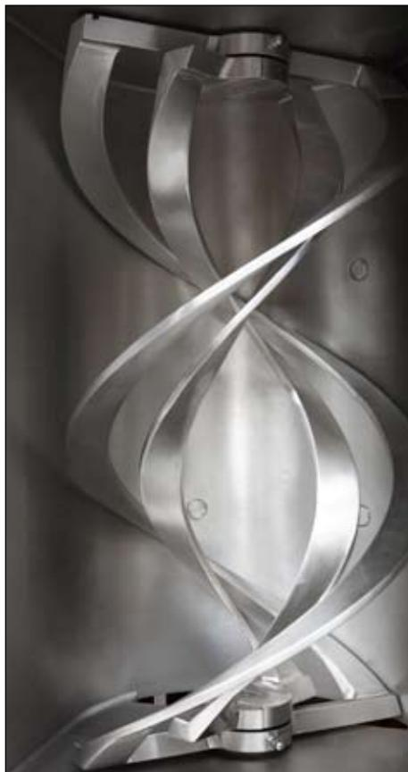
The patented Inotec Vario Mix system works without any central mixing shaft. Two horizontal interacting mixing shafts are operating in opposite directions in adjustable mixing intervals. For a better adaption to the product the mixing speed can be adjusted stepless for both spirals.
