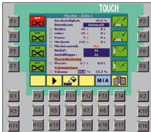
The Inotec control with touch screen panel shows the working procedure and helps to achieve the desired mixing result independently from the operator.
