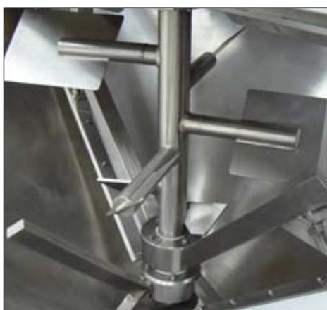
Different product buffer/pump combinations designed by Inotec are taking the product after the mixing process and convey it to filling installations. In order to avoid demixing of the mix in the buffer, Inotec offers special agitating systems to keep a gentle move of the product.
