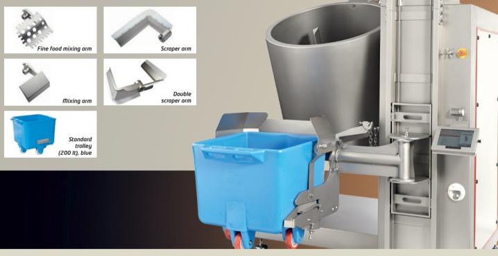
Tumbling in an upright container with an internal rotating arm offers substantial advantages: the meat is handled gently and can be processed at very low temperatures, and there is no concern of protein loss to the container wall. The two freely moving arms enable even more consistent top quality.
